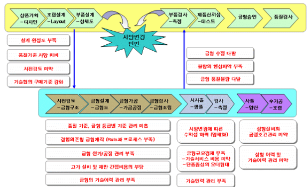
Fig. 1 Mechanism of quality problem of molds
