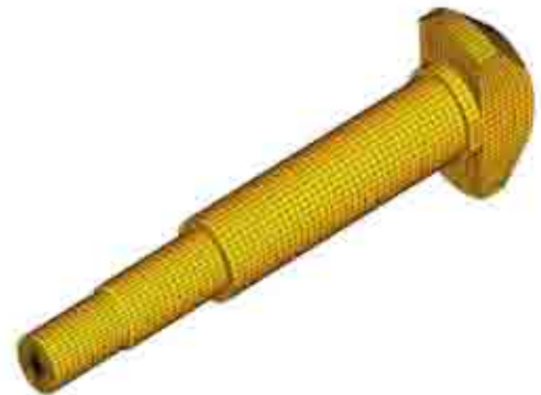
Fig. 5 FE modeling of lock
