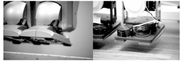
Fig. 3 Foot designs of HUBO from KAIST (left) and ARA from KIST (right) at Roboworld 2006 in Seoul
