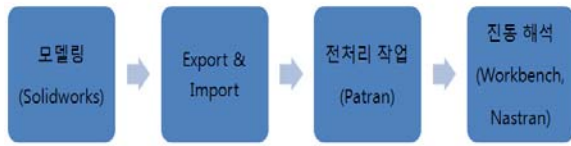
Fig. 1 Analysis Process of Hydrogen Compressor
