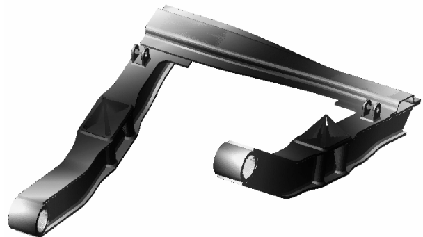
Fig. 2 The 7th mode shape of suspension frame
