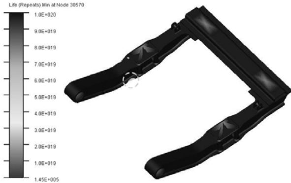
Fig. 14 Fatigue life of the suspension frame
