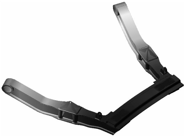
Fig. 3 The 8th mode shape of suspension frame
