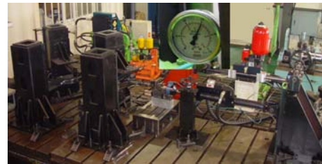
Fig. 9 The Real Plant of Dynamic Road simulator
