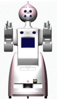
Fig.3 The Silvermate Robot having mobile base and seven joints manipulator
