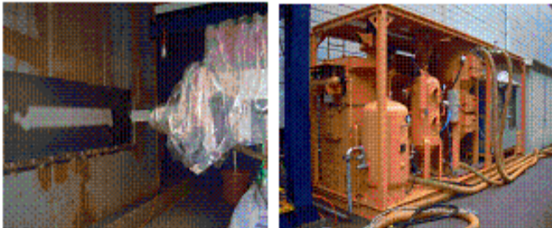
Fig. 3 Equipment for grit pneumatic conveying test (Left : 5-axis robot, Right : Grit supply system)
