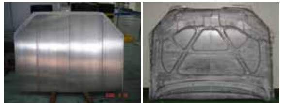
(a) TWB panel (b) press formed part
