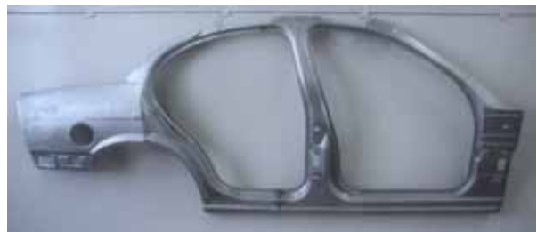
(b) Body Side Outer with TWB panel (ULSAB)
