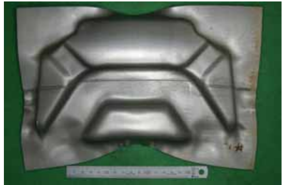
Figure 6 The result of press forming with sub-size TWB panel
