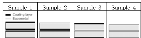
Fig. 4 Schematic of surface treatment before welding
