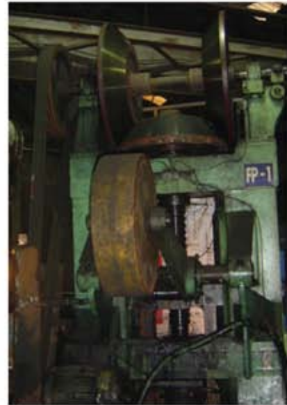
Fig. 1 150ton screw press used in experiment of the hot heading process.
