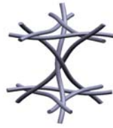
Fig. 1b and Weaved Kagome Truss Element
