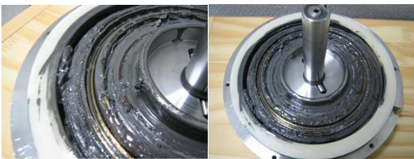
Fig. 10 Photocopy of MRF-26500 after decomposition
