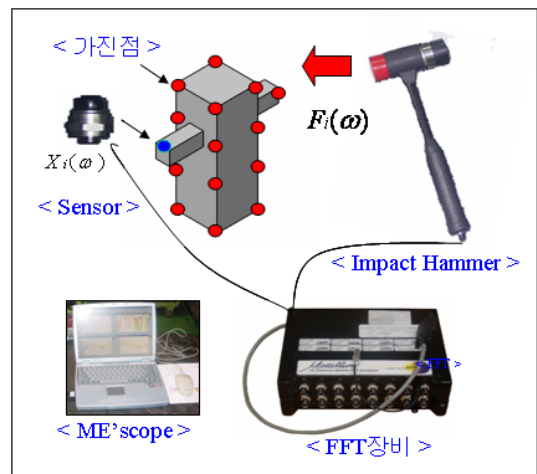
Fig. 3 Illustration of modal test setup
