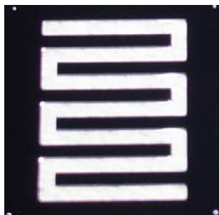
Fig. 3 Fabricated magnetostrictive actuator.
