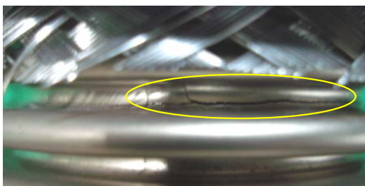
Fig. 3 Failure mode of exhaust bellows.
