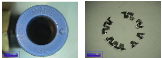
Fig. 3 Fitting failure by chuck fracture
