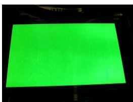
Fig.6. AMOLED display produced by SLS mixing technology.
