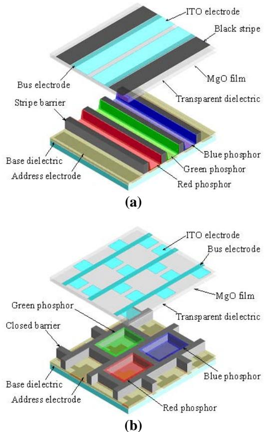
**Fig. 3. Schematics of subpixel arrangement (a) Conventional structure with stripe barrier ribs (b) SDE structure**
