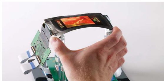
Figure 6 Flexible full color QVGA display on metal substrate made in collaboration by LG.Philips LCD and Universal Display Corporation. Vitex Systems provided the thin film encapsulation.
