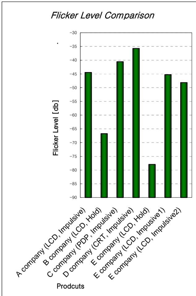
**Fig. 2. Large area flicker comparison of various displays using new metric**
