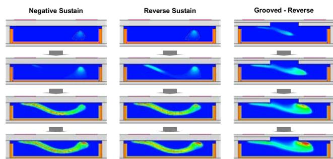
**Fig. 5. Electron density profile (Left: Negative sustain, Middle: Positive-reverse sustain, Right: Negative sustain with grooved dielectric layer)**
