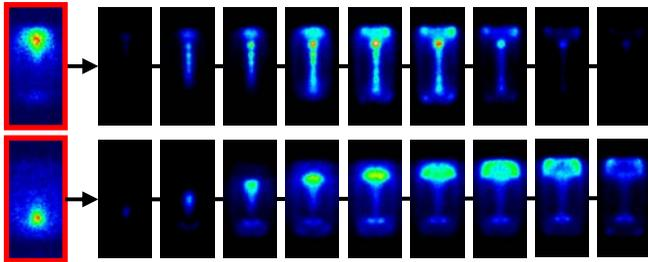
**Fig. 1. ICCD images of discharge in PDP cell (Top: Conventional dielectric layer; Bottom: Grooved dielectric layer)**
