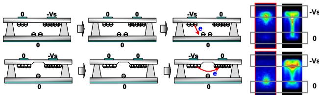
**Fig. 2. ICCD image and wall charge diagram (Top: Vertical-triggering discharge mode, Bottom: Surface-only discharge mode)**
