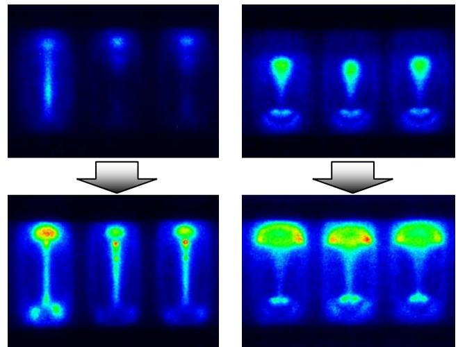
**Fig. 3. ICCD image of discharge (Left: Conventional dielectric layer, Right: Grooved dielectric layer)**
