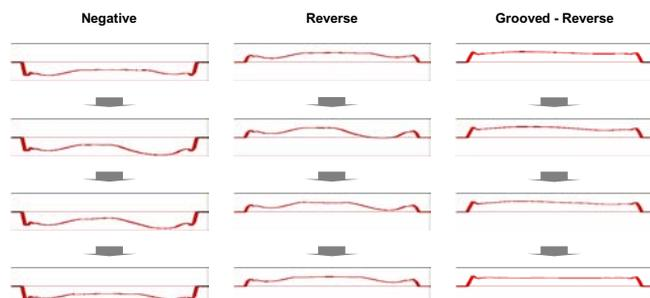
**Fig. 6. Wall charge profile on bottom substrate (Left: Negative sustain, Middle: Positive-reverse sustain, Right: Negative sustain with grooved dielectric layer)**
