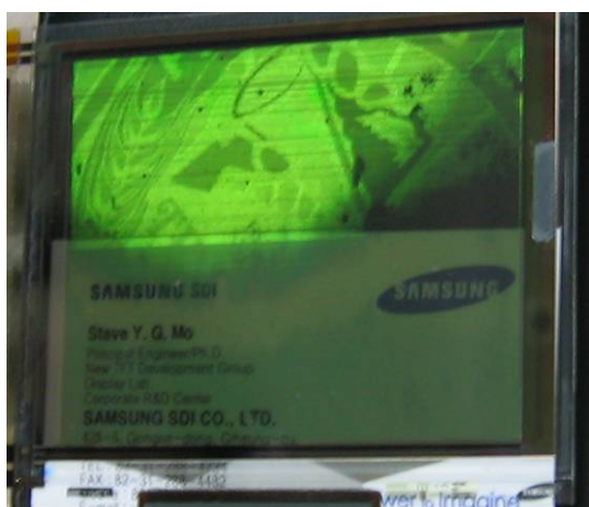
Fig. 4. Display image of transparent 4.1inch QCIF AMOLED driven by a-IGZO TFTs.
