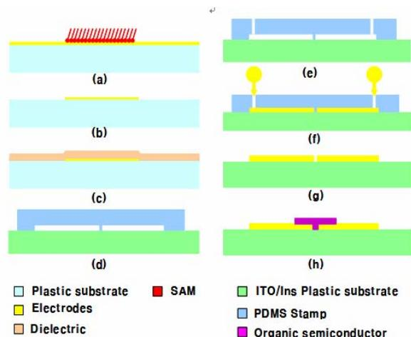
**Fig. 1. Fabrication of OTFT using microcontact printing and direct printing processes (a) Inked SAM solution on ITO deposited PEN substrate, (b) fabricated gate electrode, (c) deposited and patterned dielectric layer, (d) physical laminated on ITO and parylene formed PEN substrate, (e) fabricated injection hole, (f) injected conductive ink, (g) fabricated source and drain electrode, and (h) jetting organic semiconductor**
