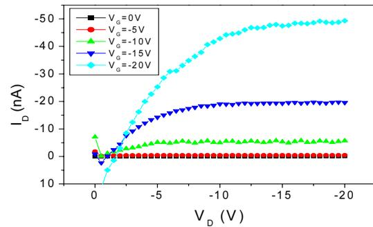
**Fig. 4.  $I_D$ - $V_D$  output characteristics of printed P3HT OTFT(W/L=500 $\mu$ m/20 $\mu$ m) (collaboration with J.B. Koo, ETRI)**
