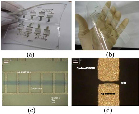
**Fig. 2. Results of OTFT fabrication: (a), (b) 5" size h-PDMS stamp and printed OTFT with channel lengths of 5 $\mu$ m, 10 $\mu$ m, and 20 $\mu$ m (width=500 $\mu$ m) on PEN substrate, (c) pentacene printed OTFT with parylene-C dielectric layer, ITO gate, and Ag source and drain electrodes using conductive Ag ink, and (d) P3HT printed OTFT on PEN substrate**
