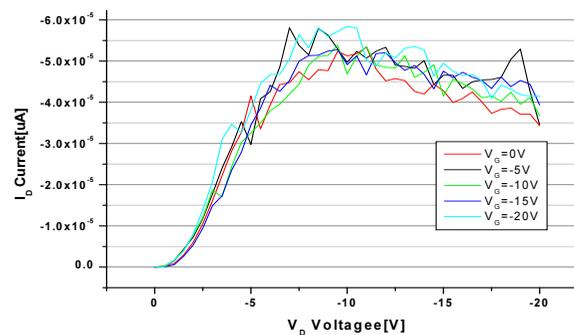
**Fig. 5.  $I_D$ - $V_D$  output characteristics of printed P3HT OTFT(W/L=500 $\mu$ m/5 $\mu$ m)**
