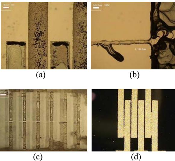
**Fig. 3. Results of failures and defects in printed OTFT fabrication: (a) infidelity, (b) leakage ink, (c) pinhole, and (d) short of channel**
