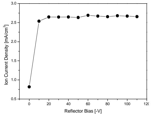
**Fig. 2. Ion current density at the reflector surface as a function of the reflector bias.**
