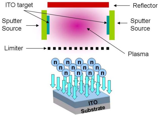
**Fig. 1. Conceptual diagram of the neutral beam source.**
