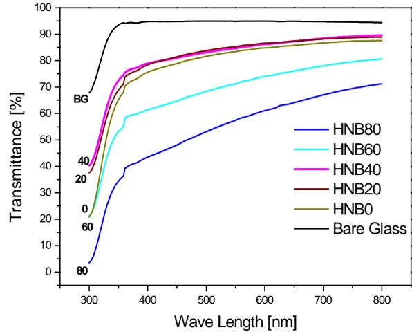
**Fig. 6. Transmittance as a function of the reflector bias.**
