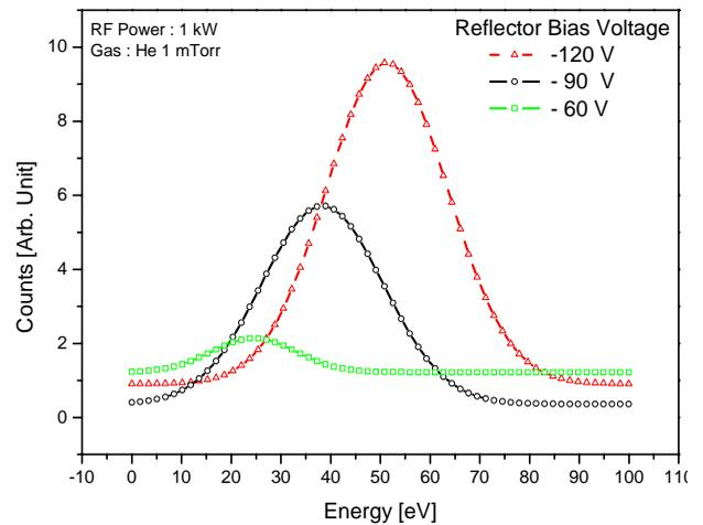
**Fig. 3. Measured neutral beam energy distribution as a function of the reflector bias voltage.**
