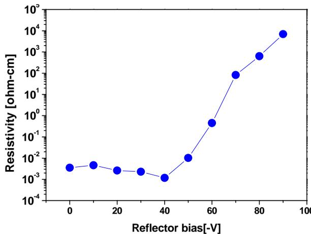
**Fig. 5. Resistivity as a function of the reflector bias.**
