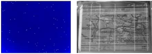
Fig. 2. (a) Drive current map for TFT array built on HS-PEN; (b) corresponding EPD build.
