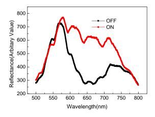
Fig. 3. The measured on/off reflectance curve of the TN modulator.
