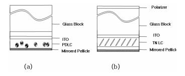
Fig.1. The cross sectional structure of PDLC modulator (a) and TN modulator (b).
