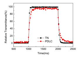
Fig. 4. The response characteristics of TN and PDLC modulators.
