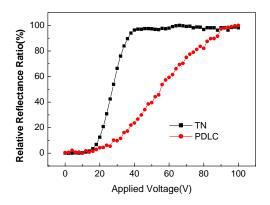
Fig. 4. The electro-optic characteristics of TN modulator and PDLC modulator.
