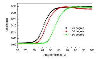
Fig. 2. Reflectance curves according to the LC twist angle.
