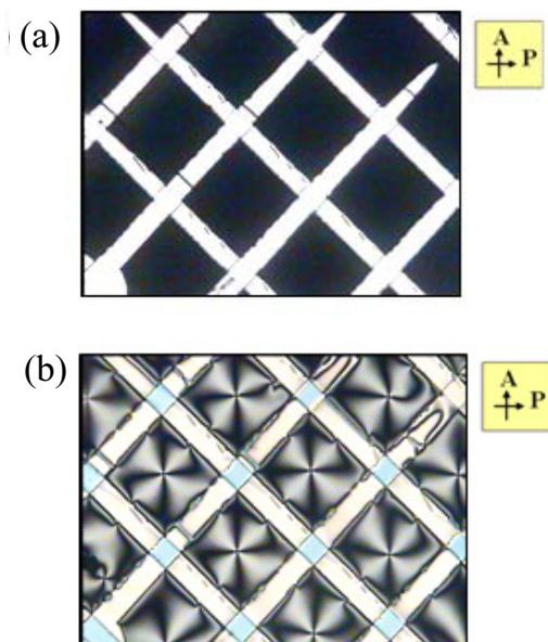
Fig. 4. The polarizing microscopic images of the LC cell fabricated with the scheme of Fig. 3: (a) field-off state, (b) field-on state.
