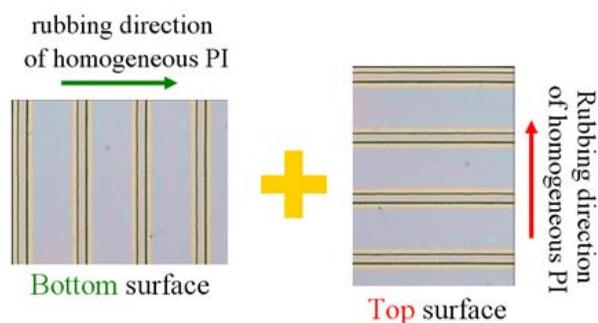
Fig. 3. The schematic diagram showing our cell assembly for producing multi-domain LC structure.
