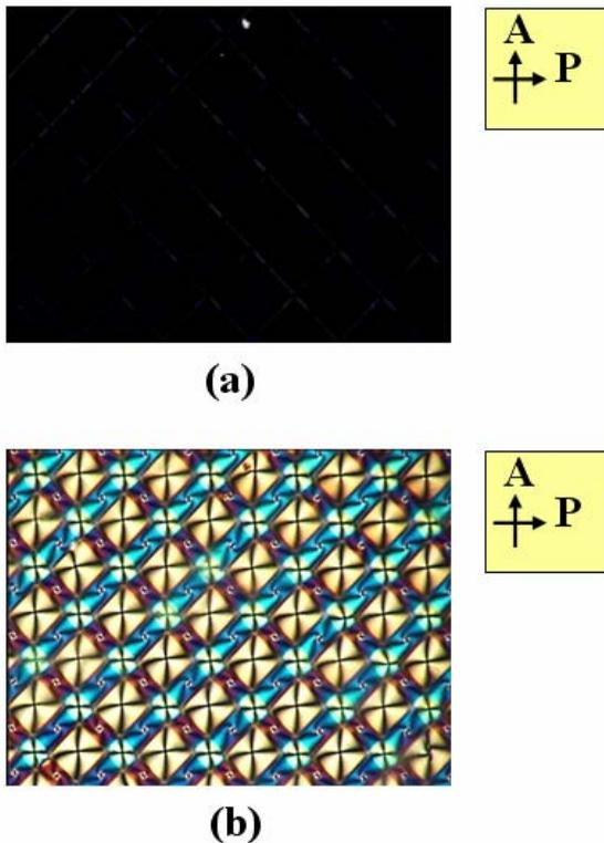
**Fig. 6.** The polarizing microscopic images of the LC textures. The LCs are aligned between a pair of the patterned surfaces with protrusions of a homeotropic PI in a periodic line shape: (a) field-off state, (b) field-on state (5 V).
