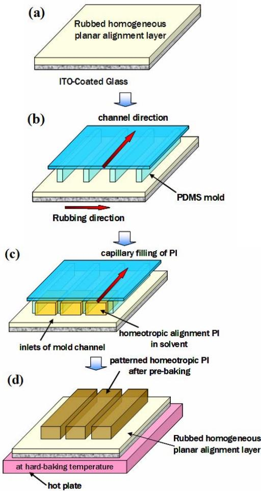
**Fig. 1. The schematic diagram of LC alignment layer patterning by the MIMIC method.**
