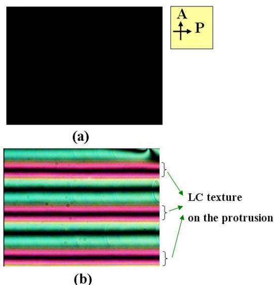
Fig. 5. The polarizing microscopic images of the LC texture. The LCs are aligned between the patterned surface with protrusions fabricated by a homeotropic PI in a periodic line shape and the non-rubbed homeotropic PI layer: (a) field-off state, (b) field-on state (5 V).
