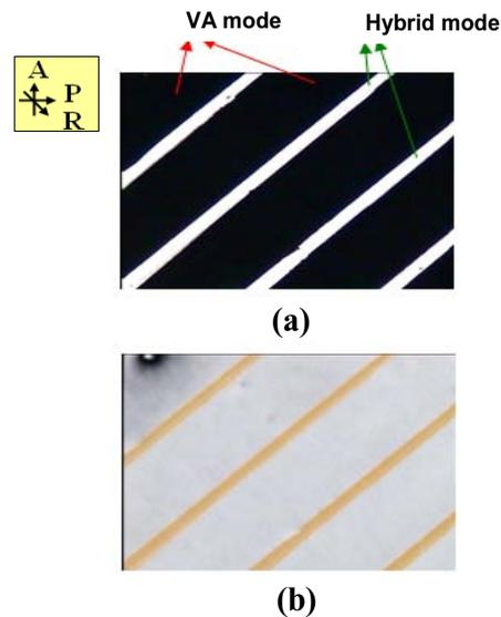
**Fig. 2. The polarizing microscopic images of the LC textures where the LCs are aligned between the patterned PI substrate (Fig. 1(d)) and the non-rubbed homeotropic PI substrate: (a) field-off state, (b) field-on state.**
