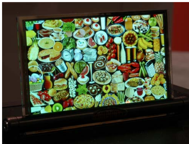
Figure 8. 4.3" WQVGA display printed by DuPont using DuPont materials and containment technology. The LTPS backplane was supplied by CMO/CMEL Corporation.
