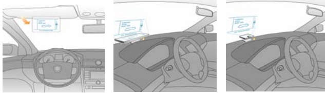
a)Direct Transparency b)Direct Reflection c) Projection
