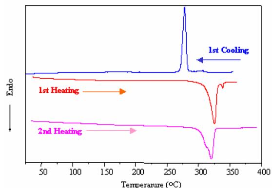
**Fig 2.** DSC Thermograms of compound with  $R = \text{H}$  (Heating and cooling rates =  $10^\circ\text{C}/\text{min}$ ).
