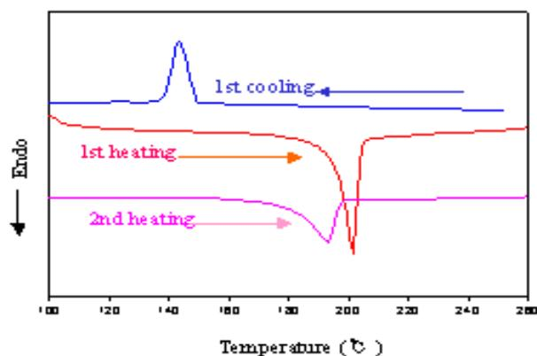
**Fig 4.** DSC Thermograms of compound with  $R = \text{OC}_8\text{H}_{17}$  (Heating and cooling rates =  $10^\circ\text{C}/\text{min}$ ).
