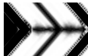
Fig. 1. Disclination of PVA Z-shape structure caused due to transmittance decrease.
