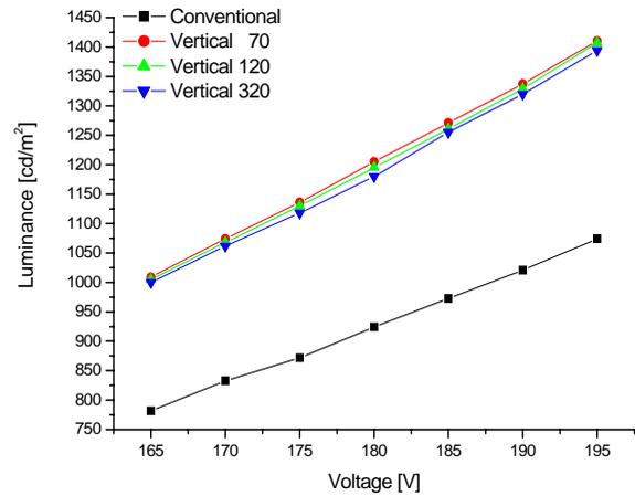
**Fig. 7. Luminance characteristics for the conventional and IBS electrode structure panels.**
