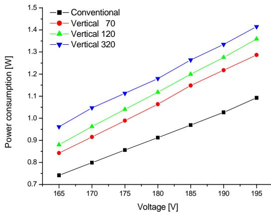
**Fig. 6. Discharge power consumption for the conventional and IBS electrode structure panels.**
