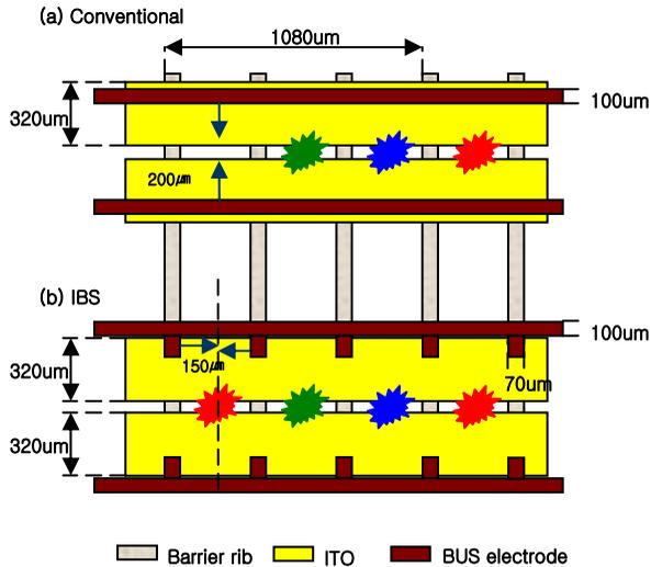
**Fig. 3. Schematic drawing of the electrical pathway in (a) conventional and (b) IBS electrode patterns.**
