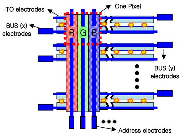
**Fig. 1.** Structure of BUS, ITO and Address electrode in Plasma display panel.
