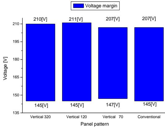
**Fig. 5. Voltage margin characteristics for the conventional and IBS electrode structure panels.**
