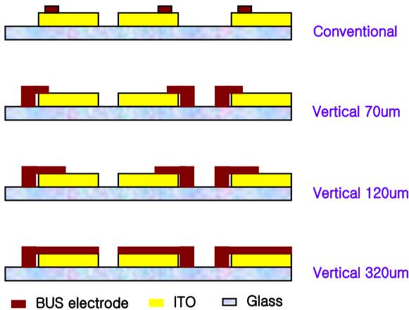
**Fig. 4. Schematic drawing of conventional and IBS electrode structure with the vertical length of 70, 120, 320µm respectively**
