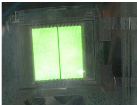
Fig. 6. Luminance of a 2-inch test panel at 185V.
