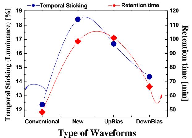
**Fig.3 Quantity of temporal image sticking and retention time for the proposed reset waveforms**
