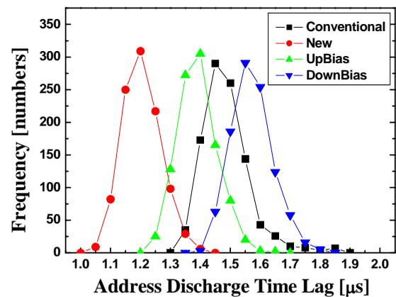
**Fig. 5** Distribution of address discharge time lag at an address pulse voltage of 65V in accordance with various reset waveforms
