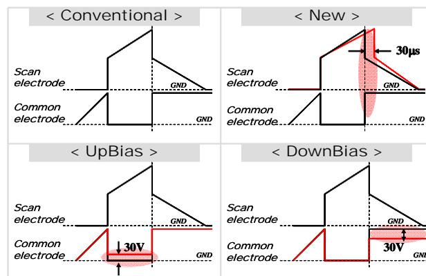
**Fig.1 Various reset waveforms for reducing black luminance**
