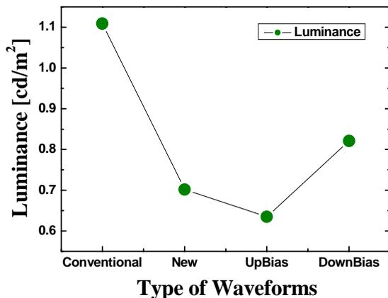
**Fig. 2 Luminance of the dark image for the proposed reset waveforms**
