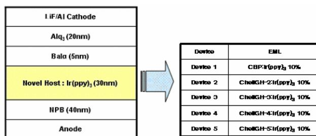
Figure 1. Device structure for evaluating novel host materials.
