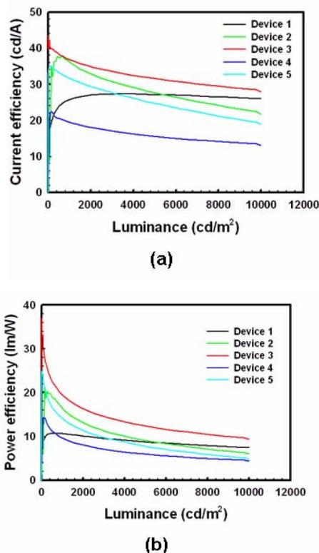
Figure 3. Device performance data of green POLEDs: (a) Current Efficiency-Luminance Characteristics (b) Power Efficiency-Luminance Characteristics
