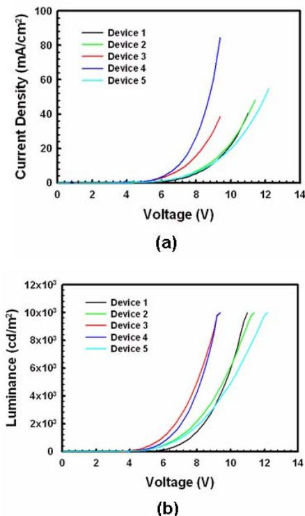
Figure 2. Device performance data of green POLEDs: (a) Current Density-Voltage Curves (b) Luminance-Voltage Curves
