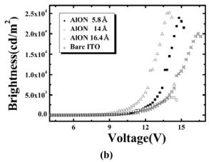
Fig. 2. (a) current density-voltage (b) brightness-voltage characteristics without and with buffer layer
