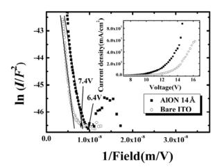
Fig. 4. Fowler-Nordheim tunneling plot with (a) and without (b) AlON treatment of the ITO surface. The curve in the close up shows the current density-voltage (*J-V*) properties of the devices
