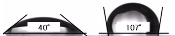
Figure 2. Contact angles of de-ionized water on PVA layer (left) and H1 layer (right). H1 layer shows much bigger contact angle than PVA layer.
