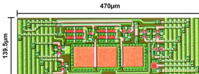
Fig. 9. Microphotograph of the proposed buffers
