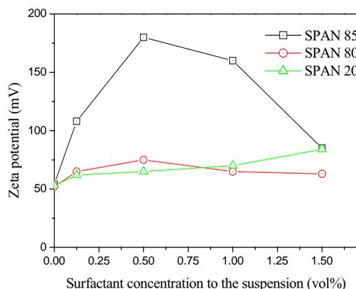
Fig. 1. Zeta potential of  $\text{TiO}_2/\text{PS}$  electrophoretic particle suspension with three different surfactants.
