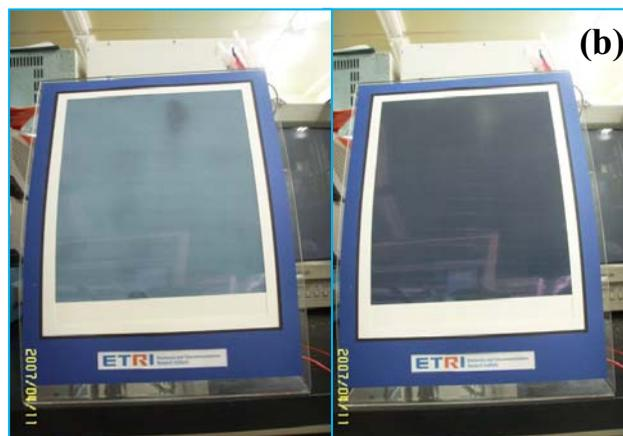
Fig. 3. Photographs of A4-sized electronic ink panel with an electrophoretic ink microcapsule diameter  $50 \pm 10$   $\mu\text{m}$  in power-on state.
