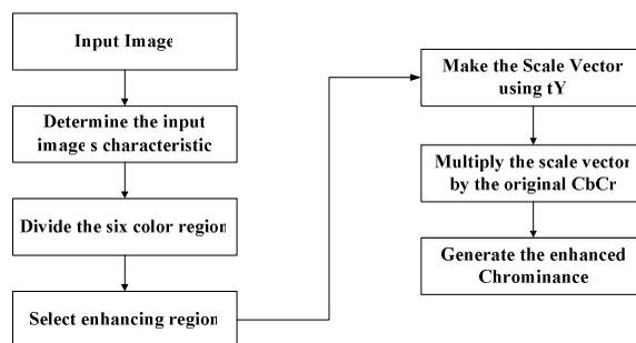
**Fig. 3. The flow chart of adaptive saturation enhancement Method**
