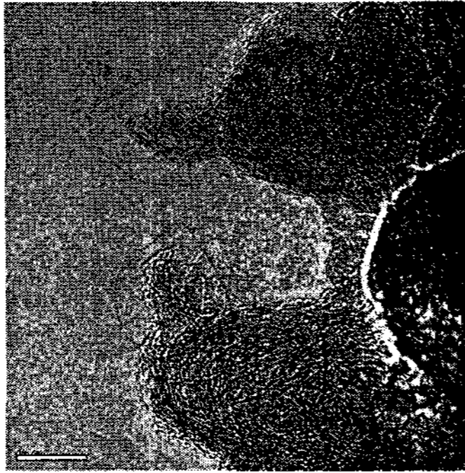
Fig. 7 TEM image of carbon black (900 °C, 1U mf , 150 g W dep. /W cat. : 0.1630 )
