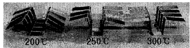
Fig. 6 Photograph of the 2D draw bending specimens in non-isothermal tests
