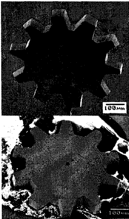
Fig. 9 Micro gear (workpiece: STS 304, \Phi_{work} = 0.4 VPt, \Phi_{tool} = 0 VPt, applied voltage: 6.5 V, pulse period: 7 \mu s, pulse on-time: 75 ns, electrolyte: 0.1 M H 2 SO 4 )
