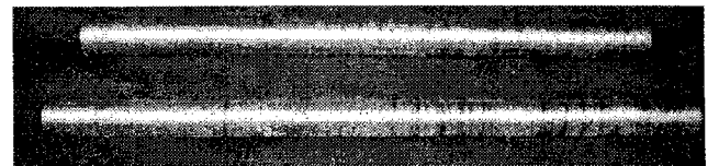
Fig. 2 Pierced pure aluminum billet by developed machine
