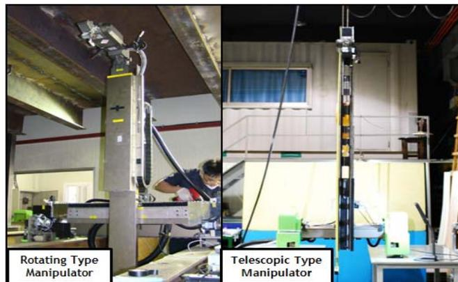
Fig. 7 Rotating and Telescopic Type blasting Robot
