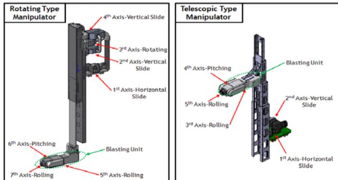
Fig. 6 Rotating and Telescopic Type Manipulator
