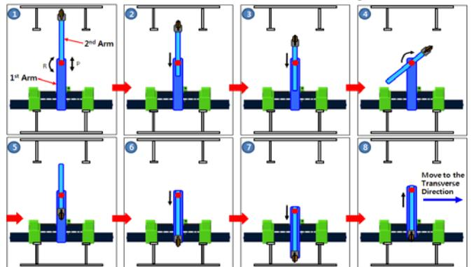
Fig. 4 Conceptual process of 'Rotating Type Manipulator' mechanism
