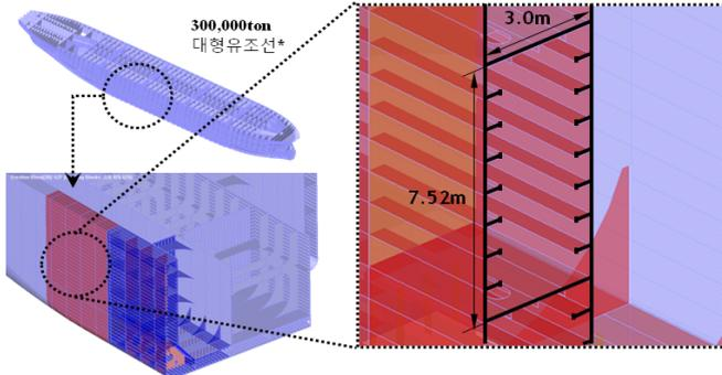
Fig. 1 Double Hull Structure of Ship
