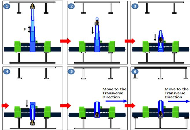
Fig. 5 Conceptual Process of 'Telescopic Type Manipulator' mechanism
