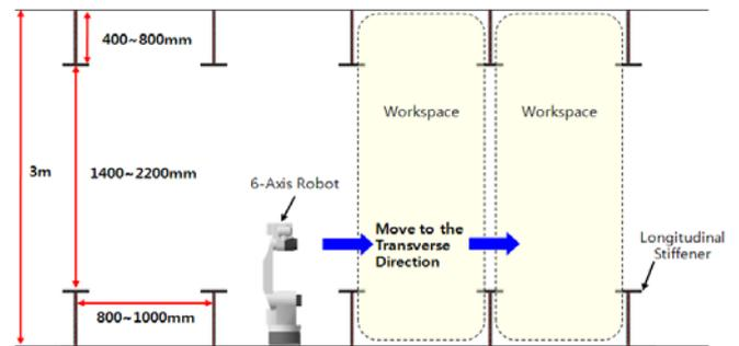
Fig. 3 Workspace of Robot in the Double Hull
