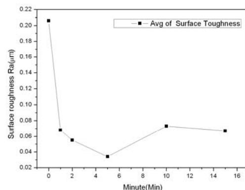
Fig. 2. Average value of surface roughness
