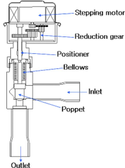
Fig. 1 Schematic of electronic expansion valve
