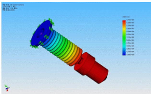
Fig. 3 Analysis result of conventional type valve
