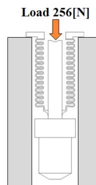
Fig. 2 Analysis model of conventional type valve
