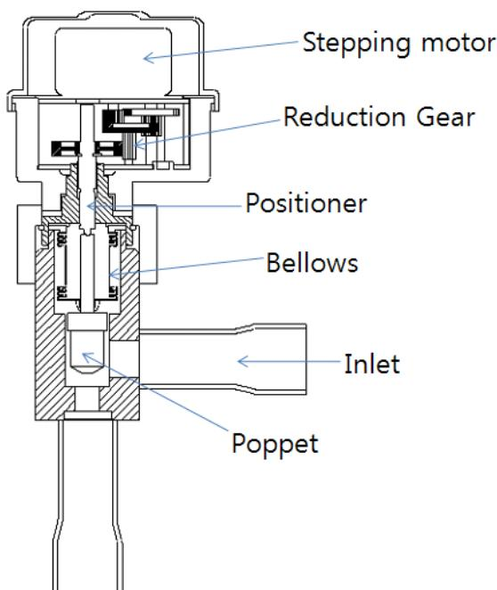
Fig. 4 Suggested model for expansion valve
