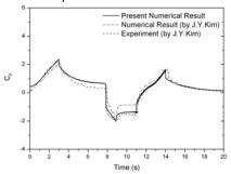
Fig.5 Comparison of  $C_p$  variations between experimental and numerical results at position of PT3.
