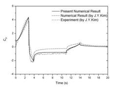
Fig.3 Comparison of  $C_p$  variations between experimental and numerical results at position of PT1.
