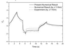
Fig.4 Comparison of  $C_p$  variations between experimental and numerical results at position of PT2.
