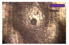
Fig. 4 Fabricated nozzle orifice through EDM
