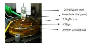
Fig. 3 EDM work on CU layer
